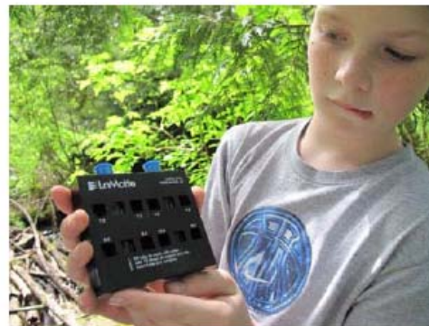
Testing the pH using the LaMotte system
